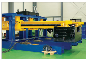
3.8ton Load Test
