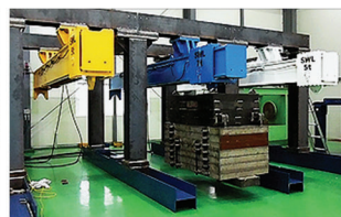
10.5ton Load Test
